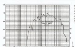
The frequency response curve is measured with the transducer located in a free-field environ-ment with a swept, sine wave signal. Input power is 1 watt and measuring distance is 1 meter. (MEASURED WITH H251 HORN)
